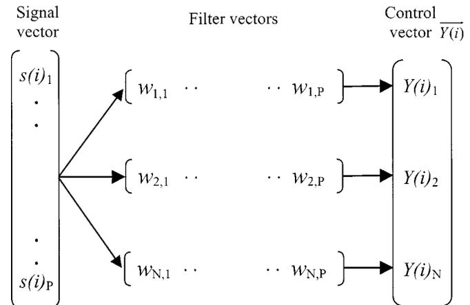
Fig. 1. Discriminatory filtering of distributed interfacial pressure data. Filtering for  $N$  fingers is shown. Filter vectors  $\vec{w}_f$  ( $f = 1 \dots N$ ), comprised of custom weights, are applied to the signal vector,  $\vec{s}(i)$ , to obtain a control vector,  $\vec{Y}(i)$ , an approximation of the intended movements.
