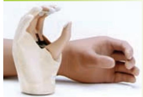
glove and a breakaway thumb for emergencies. The company has also increased the grip strength with a larger and higher torque motor. At the same time, it's also lighter than some of the older hands and only weighs about three-fourths of a pound.
