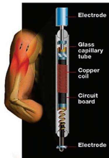
**Fig. 1.** Bionic restoration of hand mobility. This user, having nerve damage as a result of spinal cord injury, can grasp objects when his forearm muscles are stimulated with Bions. The control computer in his shirt pocket reads his intentions to grasp and activates the wire coils around his arm, to deliver electrical pulses to the Bions (brown rods).
