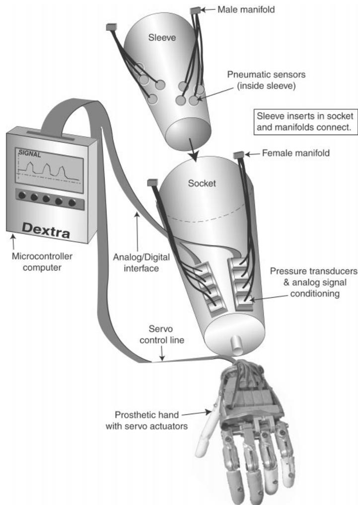
**Fig. 2.** Biomimetic *Dextra* hand prosthesis. The silicone "smart sleeve" fits snugly over the residual limb and registers 3D forces produced by muscle activity within the hard socket. The pocket computer allows the user to retrain the robotic hand for optimal performance. The hand can flex and extend all five digits in response to commands from the natural motor pathways of the user. [Figure provided by D. Curcie]
